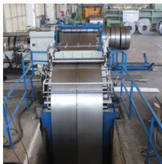
SHEET METAL SLICING LINE
