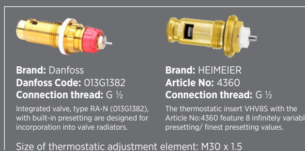
Thermostatic Valve Insert
